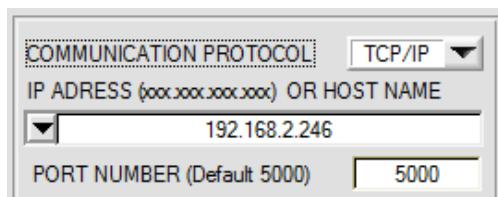
The **PORT NUMBER** for a TCP/IP connection as standard is pre-initialised as **5000**.
